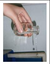
1. Rinse sample bottle with the water to be tested. Immerge the sample bottle below the surface of the water.
