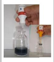
8. Add 1 drops of Reagent 5. Water turns blue or violet. Drop Reagent 4 until colorless end point.
