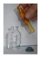
**6.** Fill the titration bottle with one full measuring tube of sample.
