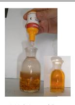
**5.** Add 4 drops of Reagent 3. Stopper the bottle. Invert the bottle several times. Flock will dissolve and the sample will turn yelloworange if oxygen is present.
