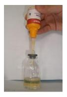
7. Add Reagent 4 by drops. Swirl to mix after each drop. Count the drops until the color become light yellow. Be carefully to hold the dropper vertically.
